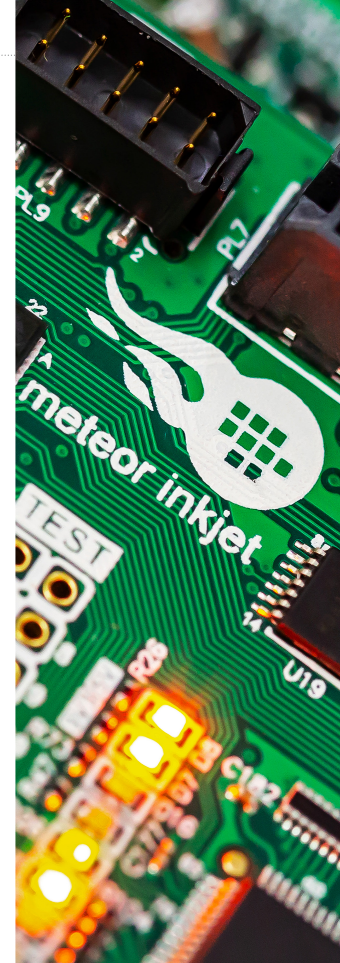
Close up example of Meteor printhead drive electronics
